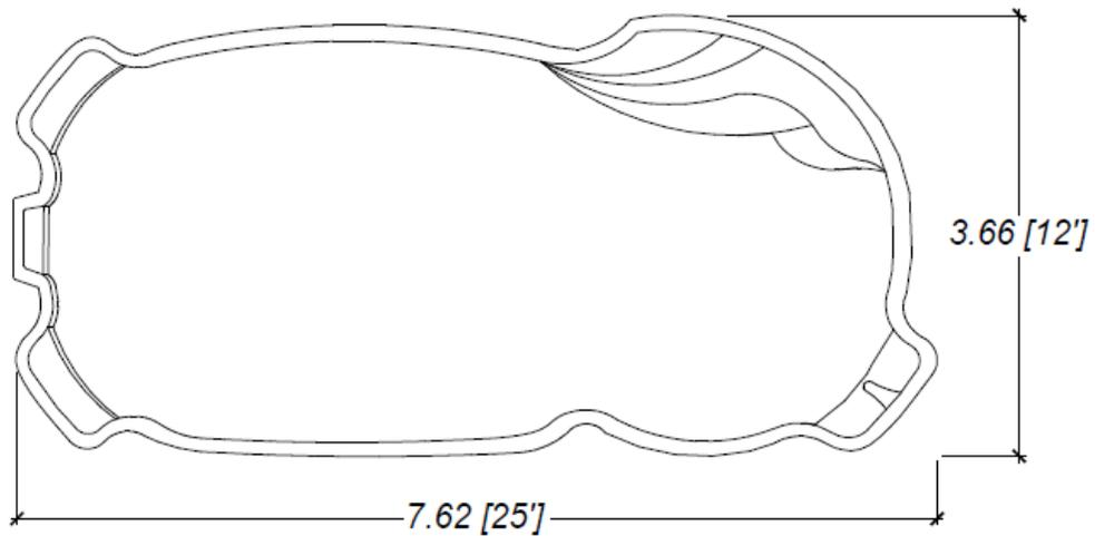
Structure de la piscine entièrement en fibre de verre. / *Structure of the swimming pool entirely in fiberglass.*
